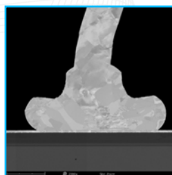
The same LED electrode after Ar-ion polishing.
