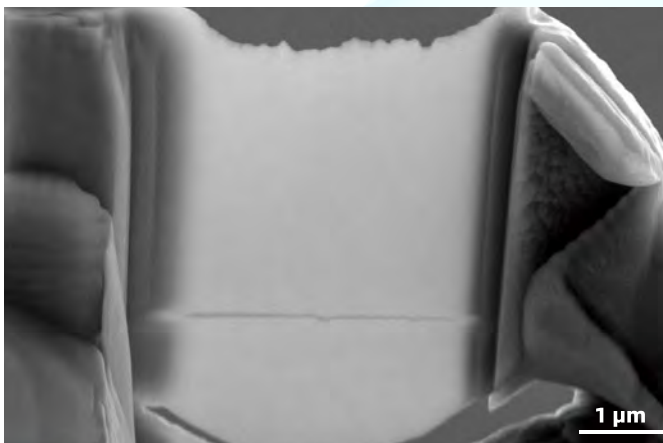
Electron image of Ferrite-martensite steel (magnetic) taken in a DB500 FIB-SEM
