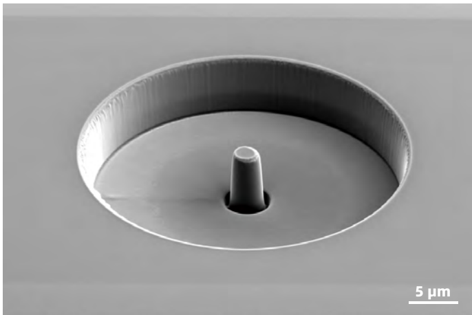
In-Situ pressure Sample Preparation
