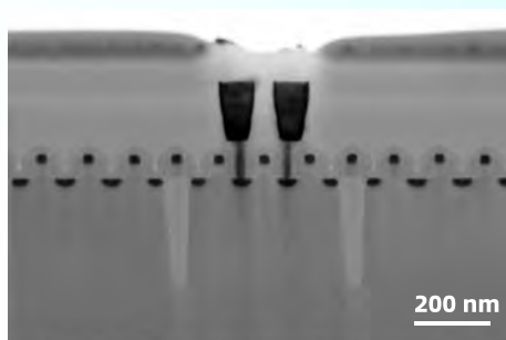
IC Chip device layer Dark-field image (STEM-DF)
