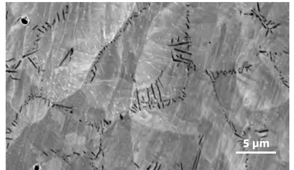
Reinforcement phases in alloy
