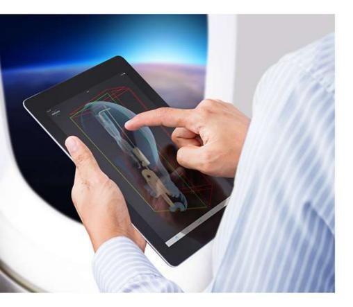
The volume rendering program CTVox also has its mobile versions, which can be freely downloaded from the AppStore for iPhone / iPad / iPod or from the Google Play for Android devices. Any 3D results obtained by SkyScan 2214 system can be sent to a mobile device for realistic visualization by real-time rendering with 3D object manipulation, virtual cutting, adjustment of opacity and colors, etc.
