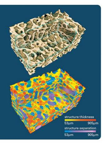
Several analysis functions in CTAn are able to provide specific morphological data based on information from half-tone reconstructed slices without image segmentation. It allows performing local 3D analysis in densely packed objects or in objects with similar X-ray absorption in different components. Such analysis is often based on 3D calculation of local signal gradients in original half-tone reconstructed data.
