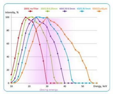
Using the X-ray interferometer for phase-contrast retrieval imposes certain restrictions on the acceptable range of X-ray energies. The system includes an X-ray source with peak energy tunable in the range 20-60 keV and an automatic filter changer with five positions to cut out low X-ray energies. Selecting the proper combination of peak energy in the source and energy filter allows tuning of a narrow band of energies according to the absorption of the object under investigation.
