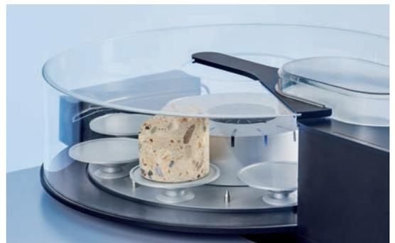
Up to 8 large samples (96 mm) or any random combination of large and small samples
