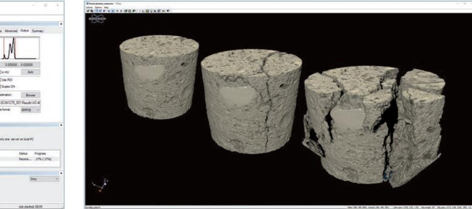
In-situ mechanical testing of a limestone plug under 0, 150 and 500 N of compression
