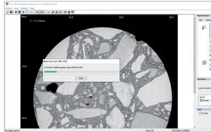
Reconstruction of a concrete core in NRECON
