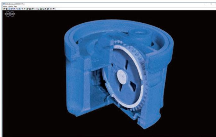
The internal components of an inhaler scanned in just 100 seconds
