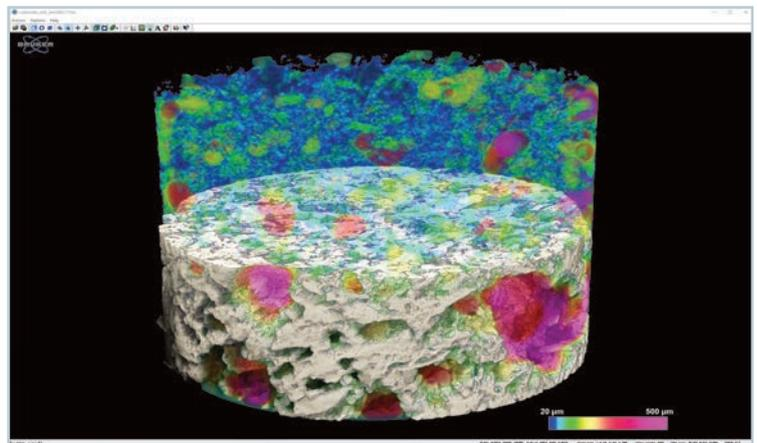
3D reconstruction of the internal microstructure of a carbonate, volume rendering with top half virtually removed overlapped with color map of local pore sizes
