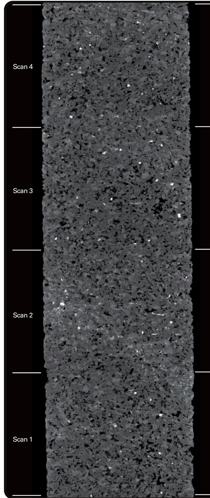
Automated stitching of multiple circular scans of a sandstone microplug
