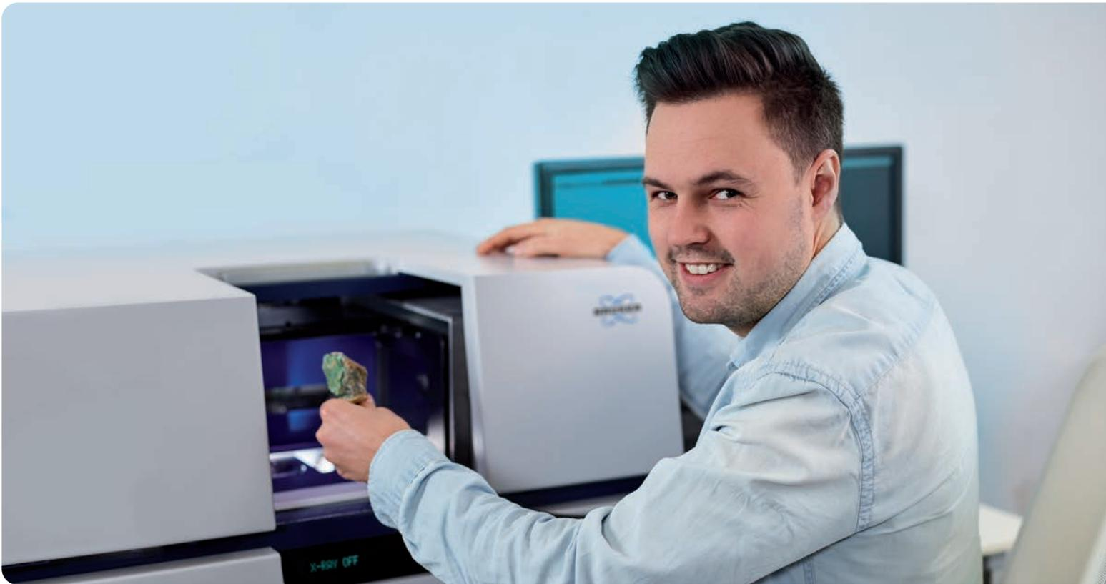
The SKYSCAN 1275 is an unparalleled desktop 3D X-ray microscope based on micro computed tomography (Micro-CT). This non-destructive imaging technology, pioneered by Bruker, uniquely provides 3D insights into samples of any material, any shape, and any size with little to no sample preparation. SKYSCAN 1275 makes this attractive technology available to everyone. This desktop instrument fits in every lab and excels in easy-of-use thanks to the high level of automation.
