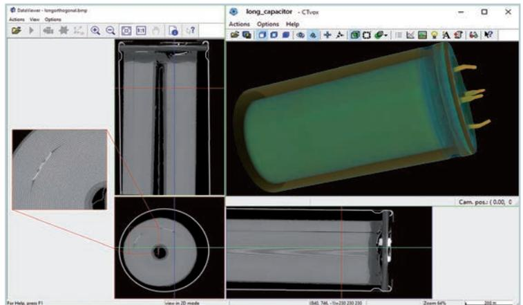
Orthogonal slices and volume render of a large capacitor.
