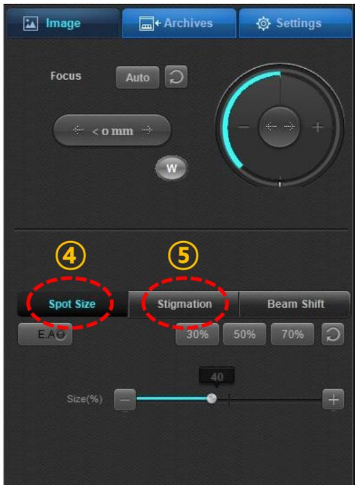
4. Resolution, contrast, and brightness can be controlled by adjusting “Quantity and Size of beam” in Spot Size mode. (Click once left button of mouse, and additional click for release)
