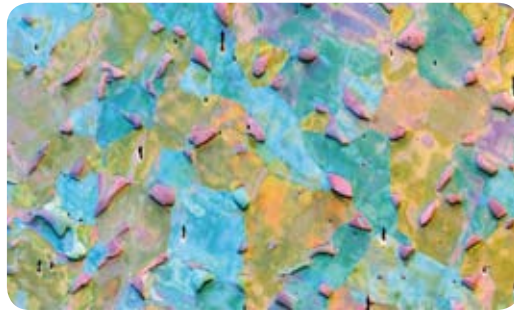
Color coded image produced by mixing the signals of the Bruker FSE detectors, showing microstructural details invisible in the greyscale image.
