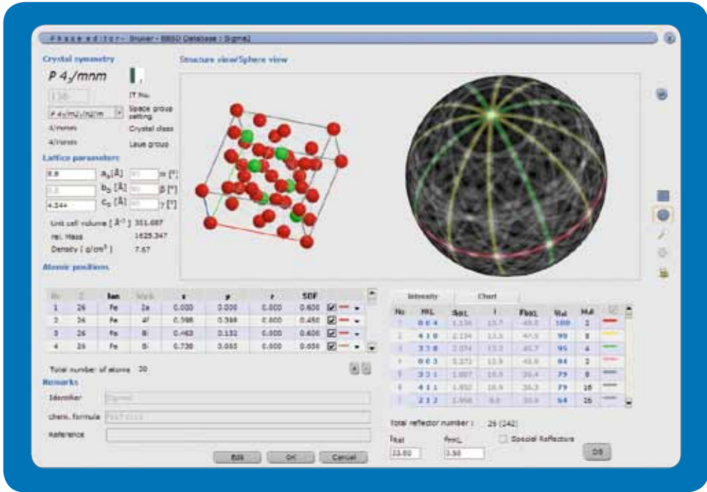
Phase editor dialog showing the crystallographic details of the "Sigma" intermetallic phase as well as the corresponding crystal structure, spherical EBSD and the reflector list.
